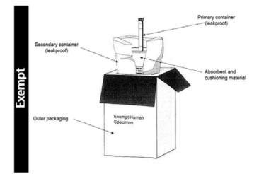
FIGURE 17-4: Illustrates the basic design of packaging system for exempt substances (Source: IATA, Montreal, Canada)
