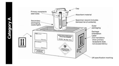
FIGURE 17-2: Example of triple packaging system for the packaging and labelling of Category A infectious substance. (Source: IATA, Montreal, Canada)
