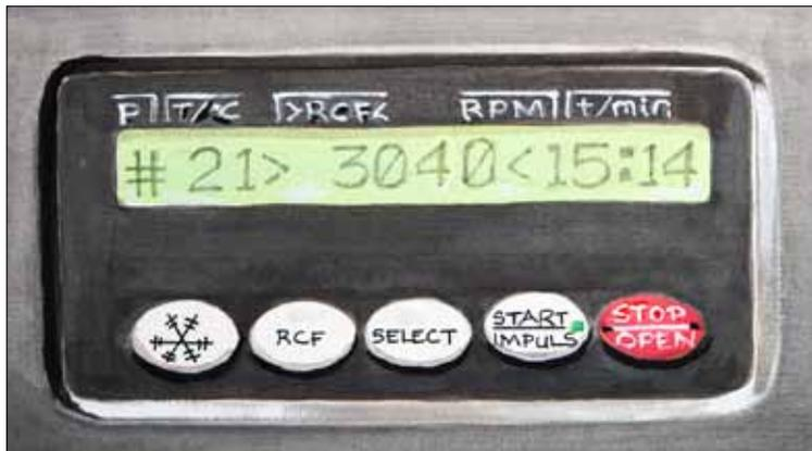
The centrifuge must be able to reach and maintain 3040 RCF (relative centrifugal force) for 15-20 minutes to sediment the majority of acid-fast bacilli
