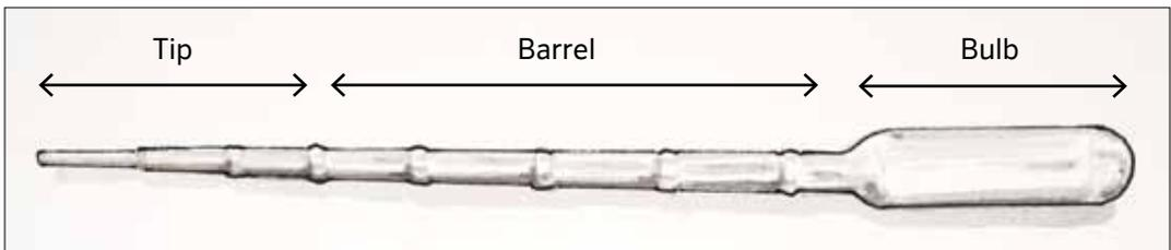
The basic structures of a disposable pipette
