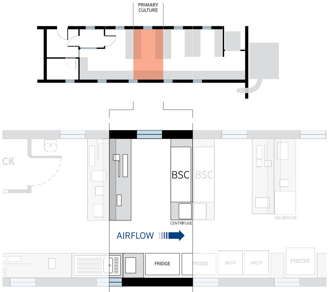
Activities generate low concentration of infectious particles. Specific equipment is required and all specimen processing must be performed within a BSC.
