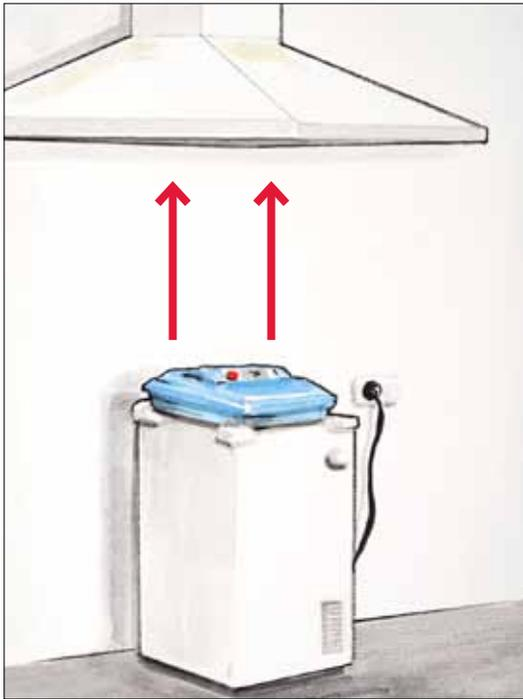
Thimble exhaust over a steam pressure sterilizer
