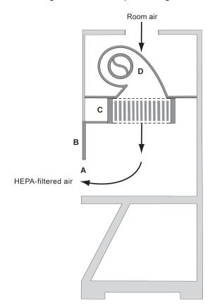
**Figure 10.** A modified containment cabinet or Class I BSC can be used for labeling infectious microorganisms with I<sup>125</sup>. (A) arm holes; (B) Lexan<sup>R</sup> hinged doors; (C) exhaust charcoal filter; (D) exhaust HEPA filter; (E) filter housing with required connection to building exhaust (see also Figure 13).
