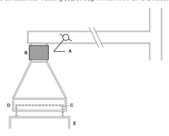
Figure 5A. The Class II, Type B1 BSC (classic design) (A) front opening; (B) sash; (C) exhaust HEPA filter; (D) supply HEPA filter; (E) negative pressure dedicated exhaust plenum; (F) blower; (G) additional HEPA filter for supply air. Note: The cabinet exhaust needs to be hard connected to the building exhaust system.
