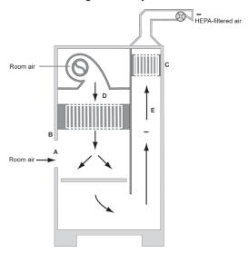
Figure 7. The tabletop model of a Class II, Type A2 BSC (A) front opening; (B) sash; (C) exhaust HEPA filter; (D) supply HEPA filter; (E) positive pressure common plenum; (F) negative pressure plenum. The Class II Type A2 BSC is not equivalent to what was formerly called a Class II Type B3 unless it is connected to the laboratory exhaust system. Note: The A2 BSC should be canopy connected to the exhaust system.
