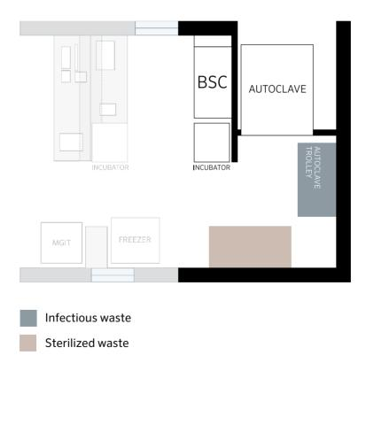
For high-workload laboratories, enough space must be provided for the storage of large loads pre and post autoclaving and for a trolley.
