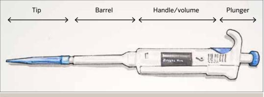
The basic structure of a micro-pipette
