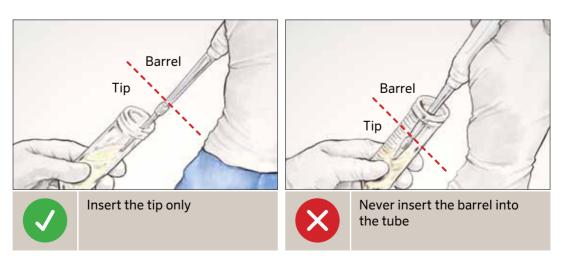
The inner diameter of a micropipette tip is narrow (<1mm diameter) and processed specimens are frequently not homogeneous in consistency and do contain portions that are >1mm. Forcing a processed specimen through a micropipette tip will block the tip and create sufficient back pressure to blow the tip from the barrel, creating infectious aerosols and a spill.
