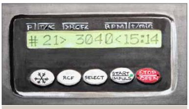
The centrifuge must be able to reach and maintain 3040 RCF (relative centrifugal force) for 15-20 minutes to sediment the majority of acid-fast bacilli
