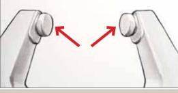
Trunnions are located on the centrifuge rotor
