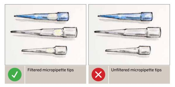
Filter tips provide effective protection from contamination of micropipettes. They prevent aerosols or liquid containing micro-organisms from entering the inner workings of the barrel.
