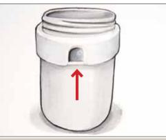
Lugs are located on each side of a centrifuge bucket
