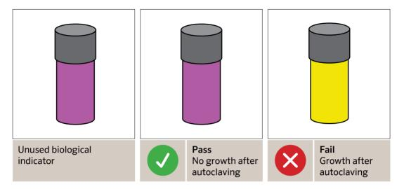
Bacterial enzyme indicators work in a similar way. They are tested post-autoclaving and once a substrate is added, a colour change indicates if the run conditions were met.
