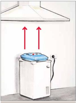
Thimble exhaust over a steam pressure sterilizer
