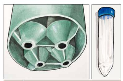
A centrifuge insert with a V-shaped base supports centrifuge tubes preventing damage
