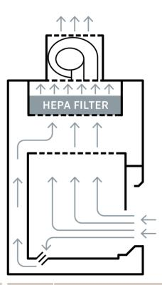
**Class 1** BSCs protect the technician but do not protect the work area against contamination because unfiltered room air is drawn over the work surface
